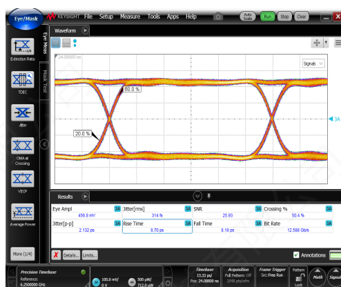
Input signal Eye amplitude = 0.45 V_{\text{pp}}
