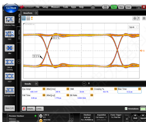
Input signal Eye amplitude = 0.45 V_{\text{pp}}
