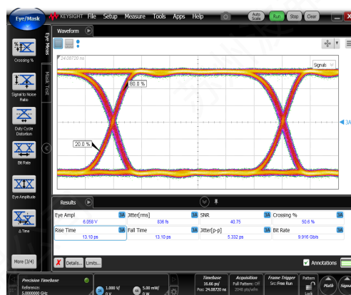
Output response Eye amplitude = 6 V_{\text{pp}}
